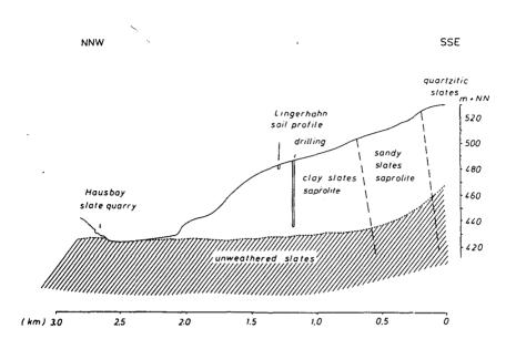
Fig. 2: Cross section of the area east of Lingerhahn village.
